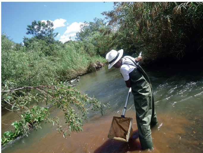
FIG. 2.2 Picture of South African Scoring System kick net during sampling, mesh size 1000 \mu\text{m} on a 30-cm square frame with stout handle. Manyame river, Zimbabwe (Photo Credit: Tongayi Mwedzi).
